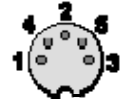
5 pin DIN female connector at the Male 5 pin DIN of MIDI cable
