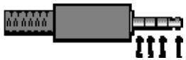
4 pin 3.5mm (2.5mm) plug connector at the iPhone (2.5mm or 3.5mm, depends on model)
